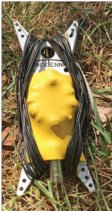
**Figure 19** — The PackTenna Mini End Fed Random Wire with an optional S-clip on the end, wrapped up and ready for a backpack. The 9:1 matching transformer is under the yellow sleeve, and coax connects to a BNC jack at the bottom.
