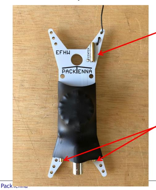
The main radiating element is soldered to the feedpoint board. If you need to replace the wire, just unsolder it and replace the wire.
