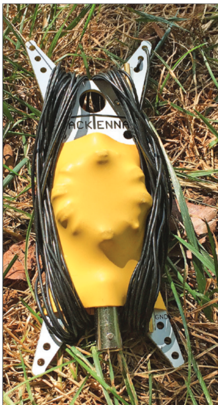
Figure 19 — The PackTenna Mini End Fed Random Wire with an optional S-clip on the end, wrapped up and ready for a backpack. The 9:1 matching transformer is under the yellow sleeve, and coax connects to a BNC jack at the bottom.
