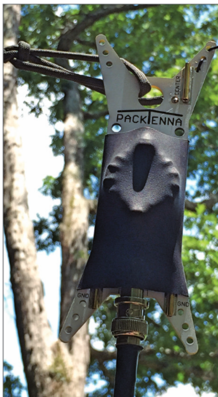
Figure 20 — The PackTenna Mini End Fed Half Wave uses the same construction as the Random Wire, but has a black sleeve and uses a 50:1 matching transformer. Note the antenna wire fed through several holes at the top right to provide strain relief for the PC board connections.
